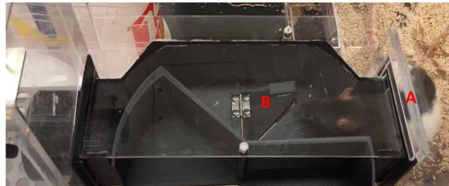
Figure 1. **A.** Sliding mechanism attaches ORD to housing cage. **B.** Pressure plate depressed (unlocked).
